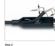
Slide the thin piece of heat shrink tubing over the headlight cable. Thread cable into junction box, strip end of conductor and tin as shown in image above.
