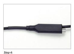
Shrink the thin piece of heat shrink tubing over the headlight cable outside the junction box. Shrink the fat piece of heat shrink tubing over the junction box itself. The junction will become particularly robust if you fill the box with hot glue before fitting the fat piece of heat shrink tubing.
